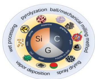
Figure 4.: Schematic illustration of the silicon–graphite hybrid anode concept. Silicon contributes high capacity, while graphite buffers expansion and maintains electronic pathways. Adapted from [1,7].
