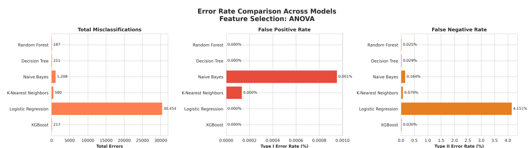
Figure 5. Error rate comparison across models showing total misclassifications (left), False Positive Rate/Type I Error (center), and False Negative Rate/Type II Error (right). Random Forest, Decision Tree, and XGBoost achieve near-zero error rates across both types. Logistic Regression exhibits extreme Type II error (4.15% FNR), missing 30,454 attacks—a critical security vulnerability.
