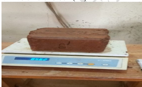
Figure 8: Weighing of compressed laterite interlocking blocks
