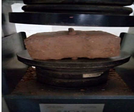
Figure 9: Tensile test of compressed laterite interlocking blocks.
