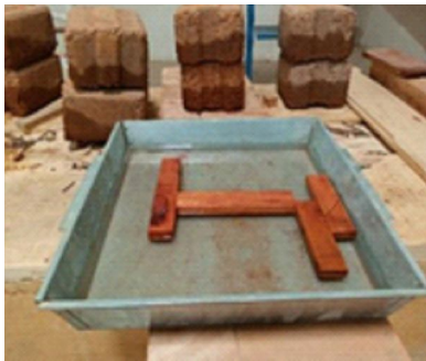
(a). Water absorption set-up
