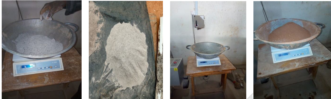
Figure 5: Batching of the various aggregates in percentages.
