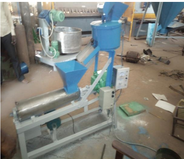
Figure. 3: Assembly work of the groundnut roasting and peeling machine
