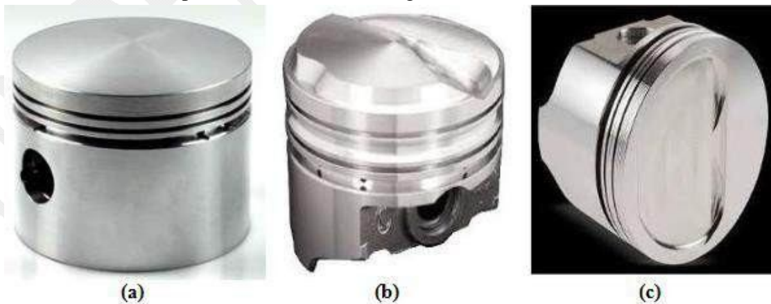
Figure 2: Piston heads (a) Flat head (b) Concave head (c) Convex Piston (Silva et al., 2013)
