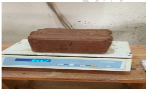
Figure 8: Weighing of compressed laterite interlocking blocks
