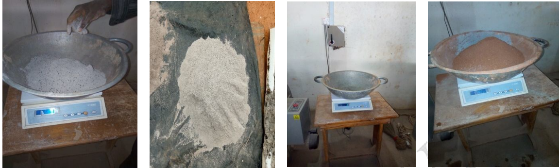
Figure 5: Batching of the various aggregates in percentages.
