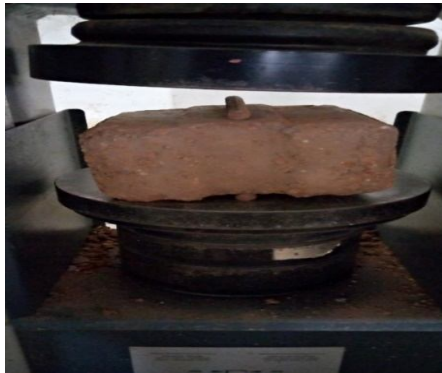
Figure 9: Tensile test of compressed laterite interlocking blocks.
