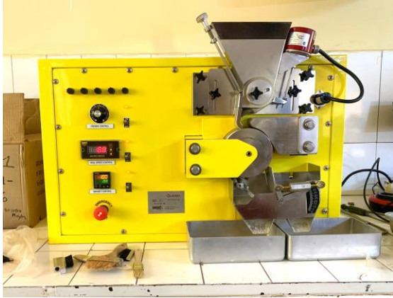
Figure 5. Outotec high-intensity magnetic separator
