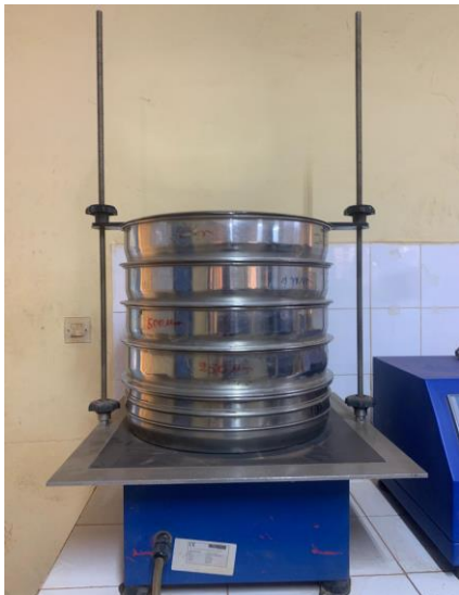
Figure 2. Sieve column mounted on an automatic sieving machine
