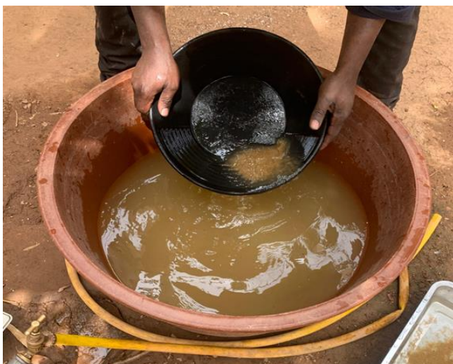
Figure 3. Gravimetric separation by panning
