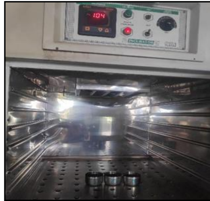
Plate. 3. measurement of moisture content of sample using hot air oven
