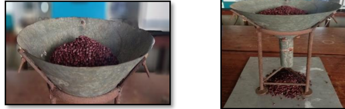
Plate. 7. Measurement of angle of repose of groundnut seeds
