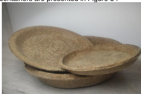
Figure 3. Samples of biodegradable containers made by pressing on the basis of wheat bran.
