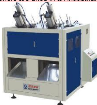
Figure 1. ZDJ-400 automatic machine for the production of biodegradable containers .
