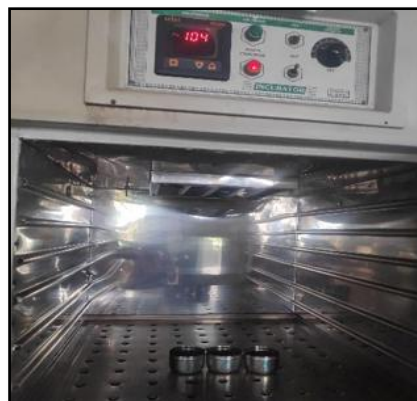
Plate. 2. measurement of moisture content of sample using hot air oven
