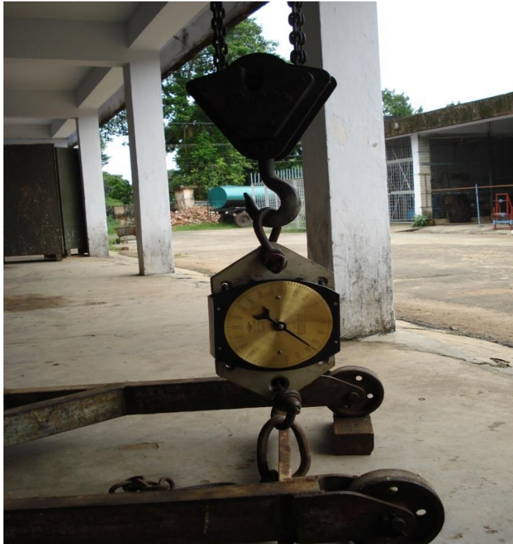
Fig. 4. Measurement of dynamometer spring deflection
