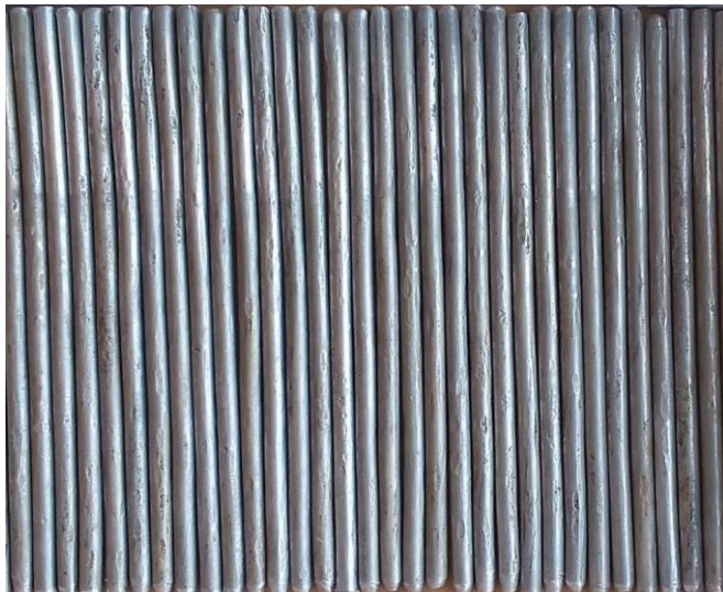
Plate 5: Heat Transfer Internal Cylindrical Fins ( \text{Ø}5 \times 140 \text{ mm} )
