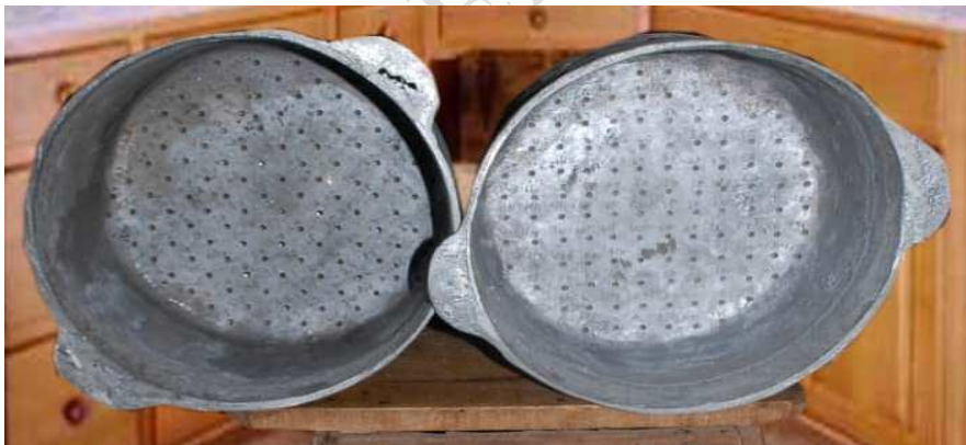
Plate 4: 7-litre EABPs Showing the Internal Cylindrical Fins' Potential Placement Locations
