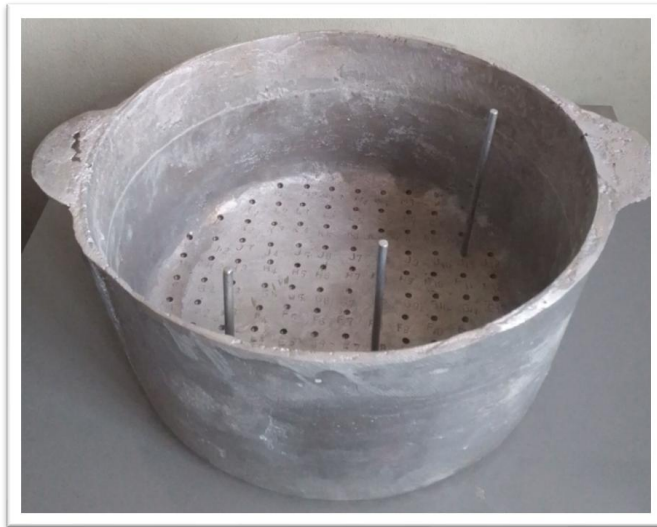
Plate 6: The EABP Incorporated with Xmas Tree Rule Using 3-Internal Cylindrical Fins
