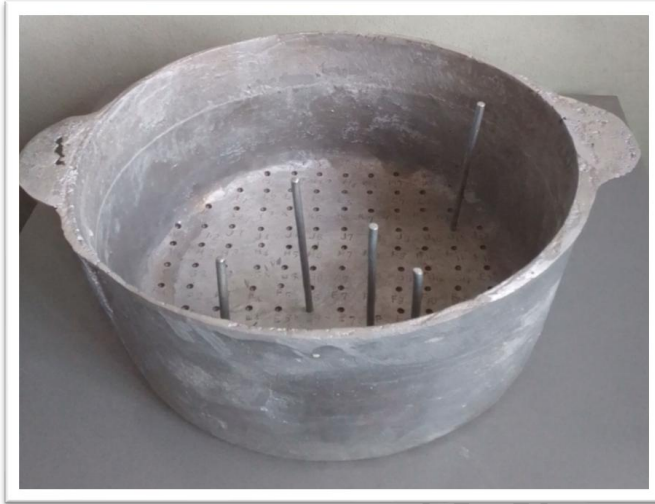
Plate 7: The EABP Incorporated with Xmas Tree Rule Using 5-Internal Cylindrical Fins
