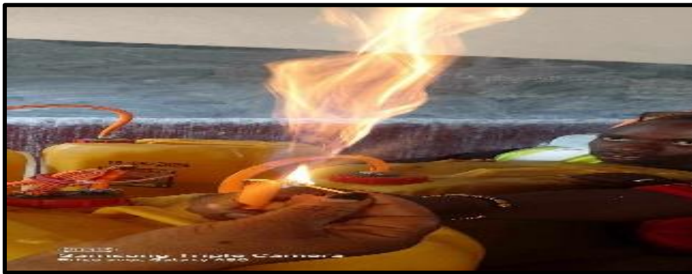
Figure 8: The image of a combustibility test of biogas produced from the anaerobic fermentation of plantain leaves.
