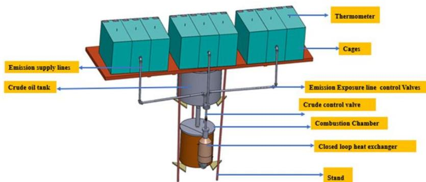
**Figure 1:** Isometric model of locally fabricated artisanal refinery combustion chamber
