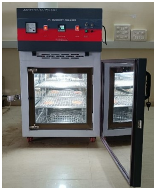
Figure 2: Dynamic temperature-humidity chamber
