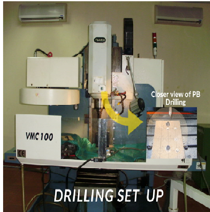
Figure 2 Experimental setup and Drill bit used
