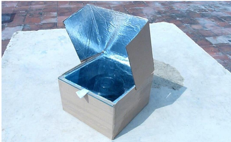
Figure 6 : Solar box type Dimensions (235mmx235mmx140mm)
