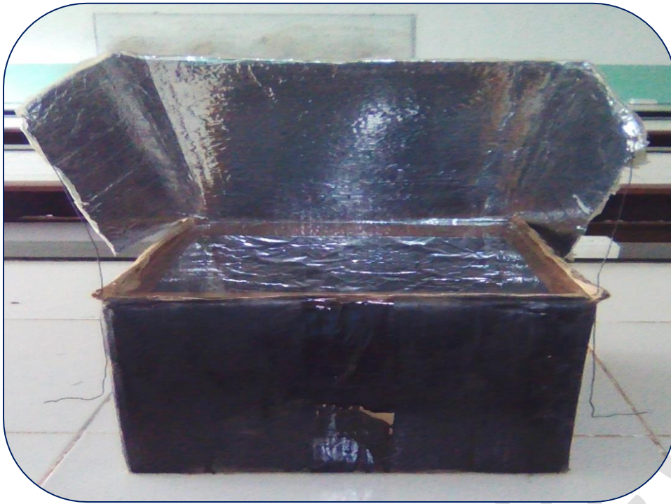
Figure12: Solar cooker box type. Dimensions (50cm x 40cm x 30cm)
