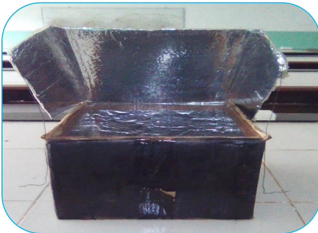
Figure 7: Solar cooker box type. Dimensions (50cm x 40cm x 30cm)
