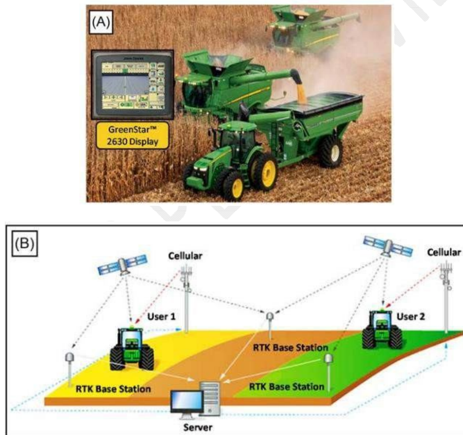
Fig. 2: (A) Combine harvester equipped with an Auto Trac system using a GreenStar 2630 Display for the guidance system and a host of other precision farming applications, developed by John Deere and (B) Mobile RTK corrections using 3G/4G communications [31].
