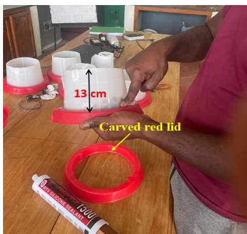
Fig 1: Flux chamber construction
