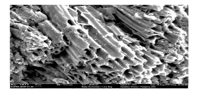
Fig. 4. Scanning Electron Microscope image of activated carbon (AC) pore topography
