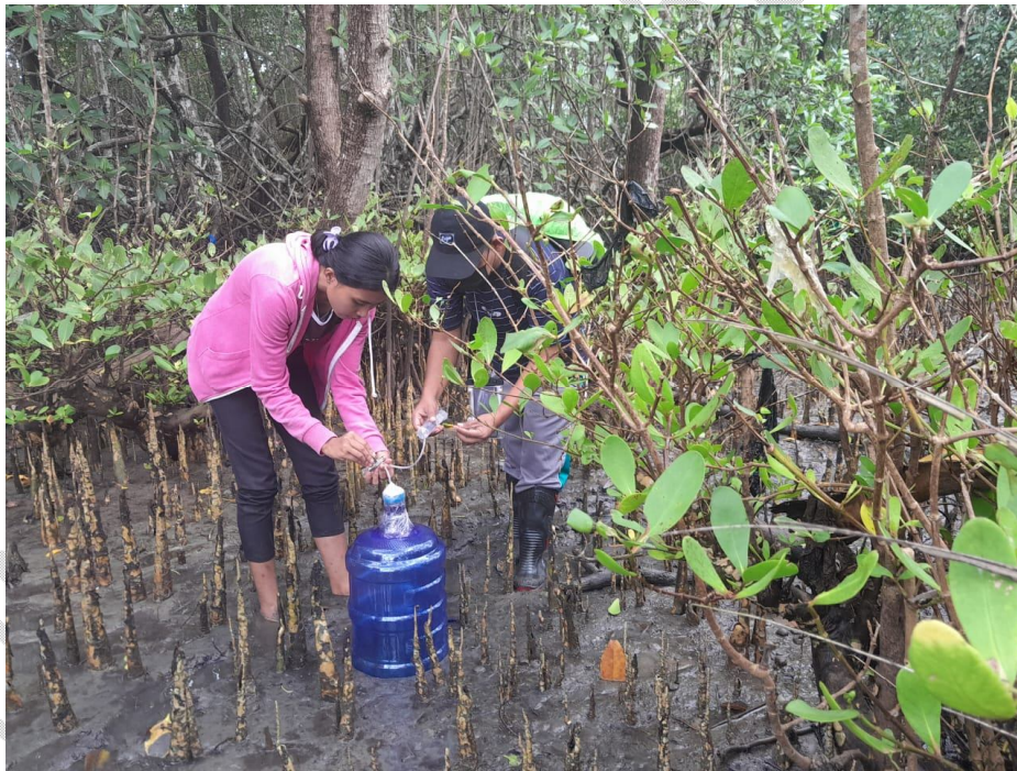
Figure 2. Gas Sampling Using a Cylindrical Chamber
