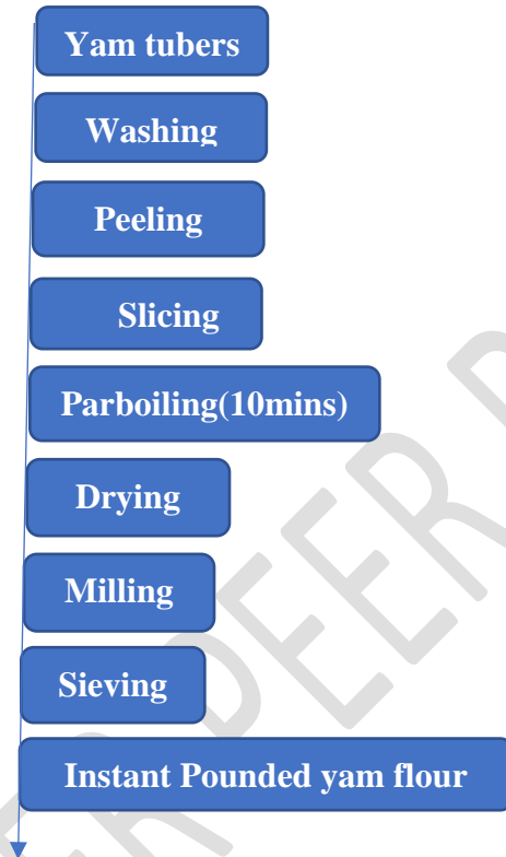
Fig 2: Flow chart for the production of instant pounded yam
