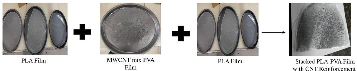
Fig.3. A) Stacked PLA-PVA Film, B) Stacked PLA-PVA with MWCNT reinforcement
