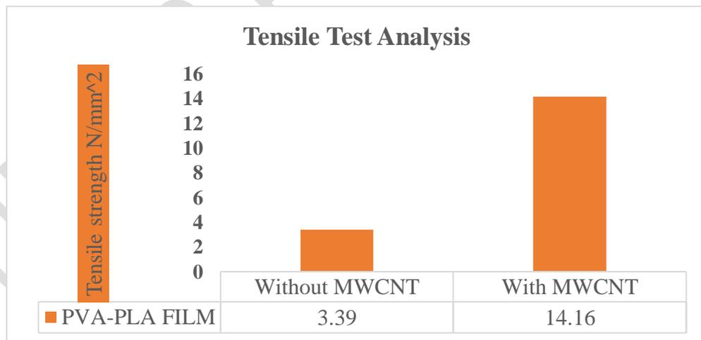
Fig. 6. Tensile strength comparison.
