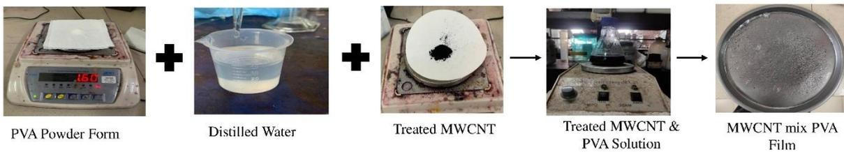
Fig. 2. A) Treatment of MWCNT, B) MWCNT Reinforcement PVA Film
