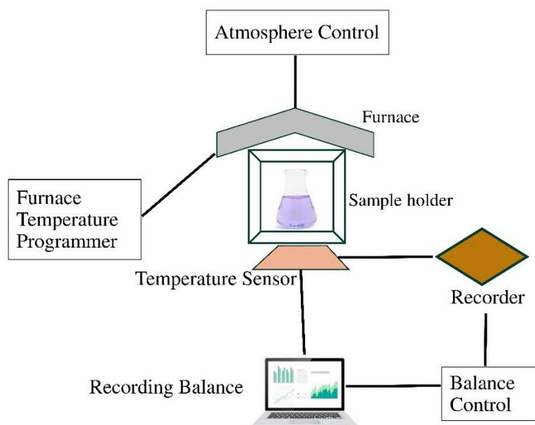
Fig.4. Block diagram of TGA machine [35]
