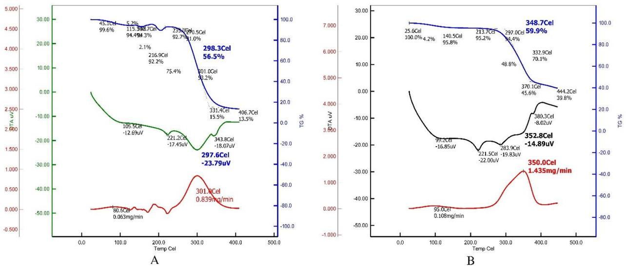
Fig.8. A) TGA/DTG curve for without MWCNT reinforced film, B) TGA/DTG curve for with MWCNT reinforced film.
