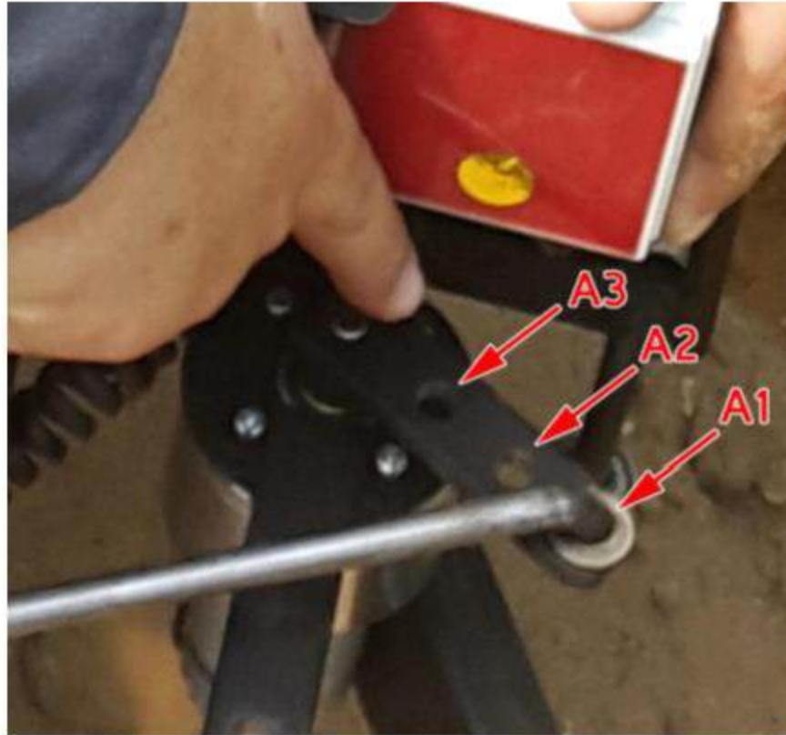
Figure 9 : Three holes on the small arm of the machine
