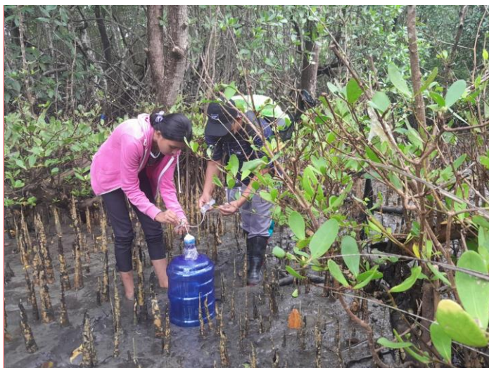
Figure 2. Gas Sampling Using a Cylindrical Chamber
