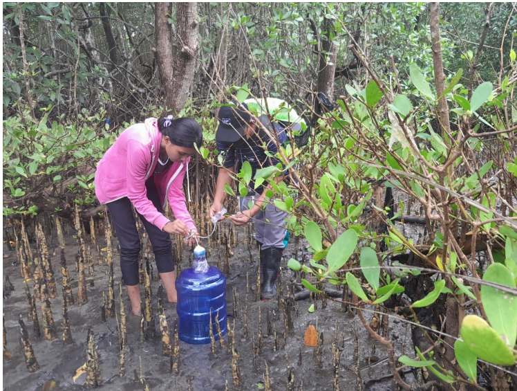
Figure 2. Gas Sampling Using a Cylindrical Chamber
