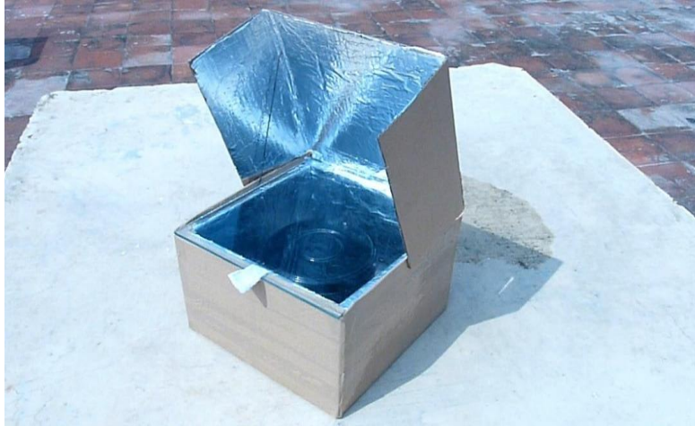
Figure7: Solar box type (accessed 25/05/2016). Dimensions (235mmx235mmx140mm)
