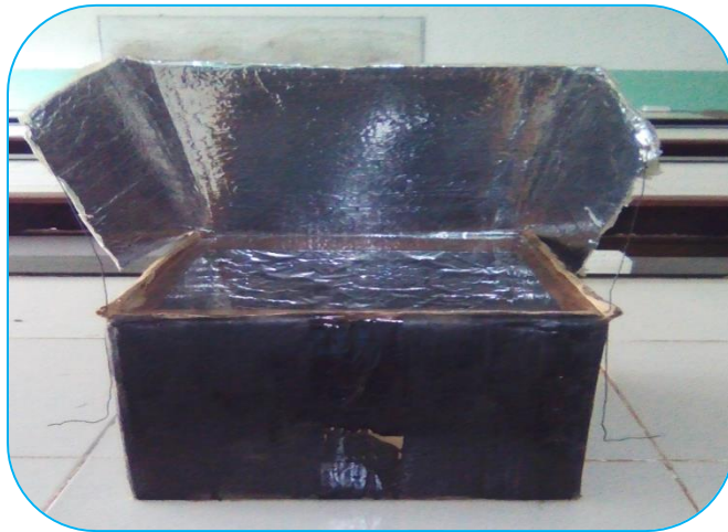
Figure8: Solar cooker box type. Dimensions (50cm x 40cm x 30cm)
