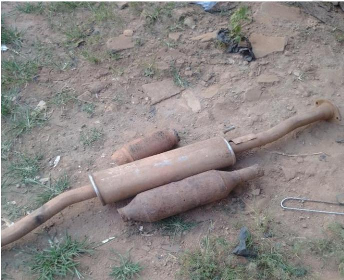
**Figure 1:** Exhaust System Parts for failure analysis
