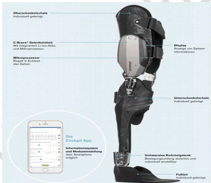
Figure 9: C-Brace: Computer-controlled leg orthosis From Ottobock
