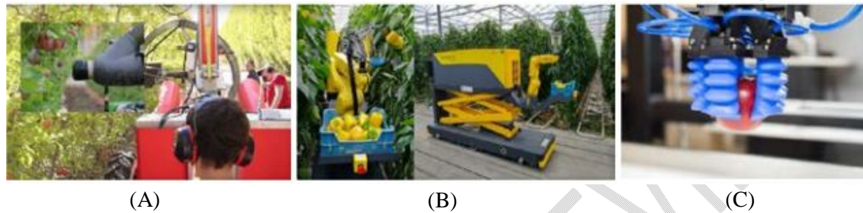
Fig.6 (A) Apple vacuum-harvesting robot, developed by Abundant Robotics [6], (B) Sweet pepper harvesting robot, developed by Sweeper [5], and (C) Robotic grippers and the control unit, developed by Soft Robotics [25].
