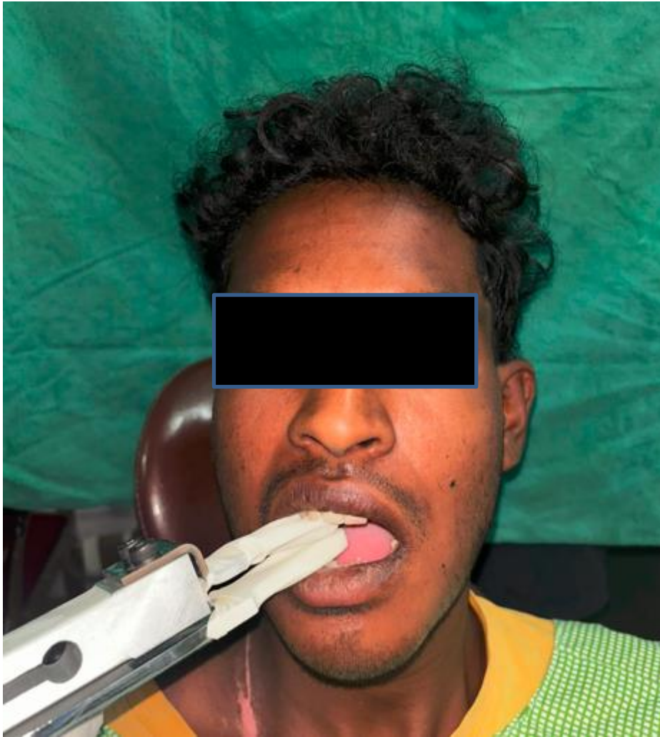
IMAGE 1: PICTURE DEPICTING USE OF BITE FORCE DEVICE FOR MEASURING THE BITE FORCE.
