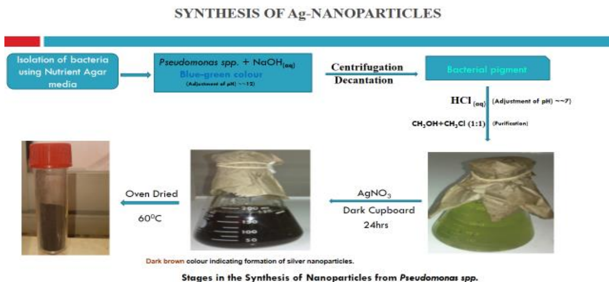
Figure 1: Process flow in the extraction and synthesis of Ag NPs modified from Jimoh et al. , (2022)
