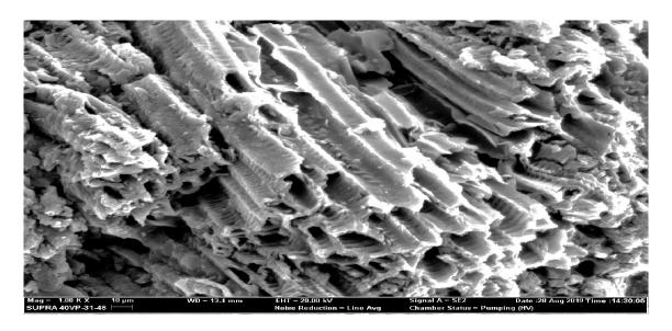
Fig. 4. Scanning Electron Microscope image of activated carbon (AC) pore topography
