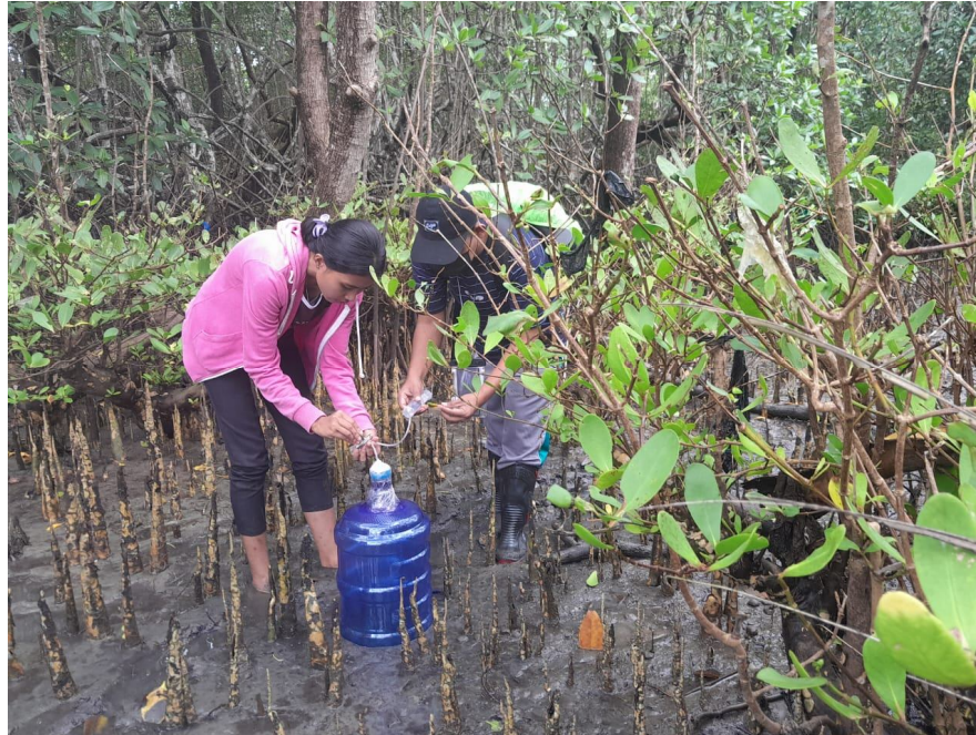
Figure 2. Gas Sampling Using a Cylindrical Chamber
