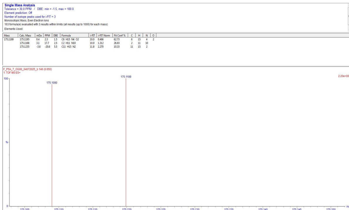
Fig. 10. Mass Spectra of L-Arginine after FDC experiments, ESI set in positive mode (174.204 +1), Retention Time (minutes) set at 0.64 ± 2.00, 174.204 +1 at 175.119 Da.
