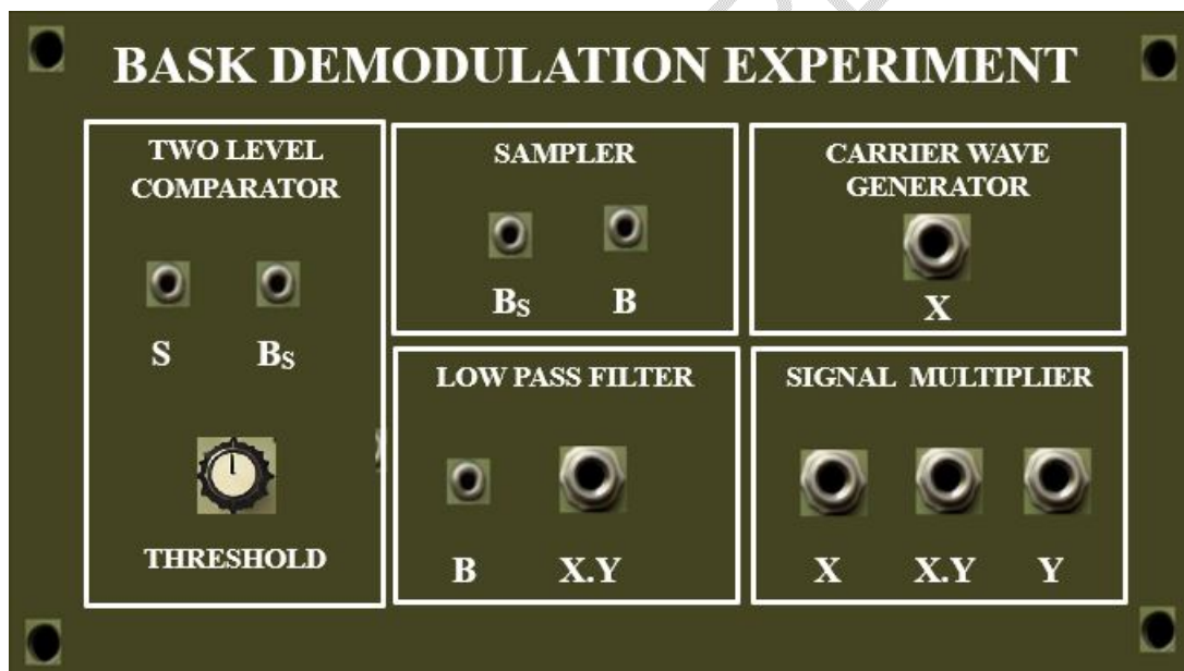
Fig.8. Experimental Equipment for BASK Demodulation
