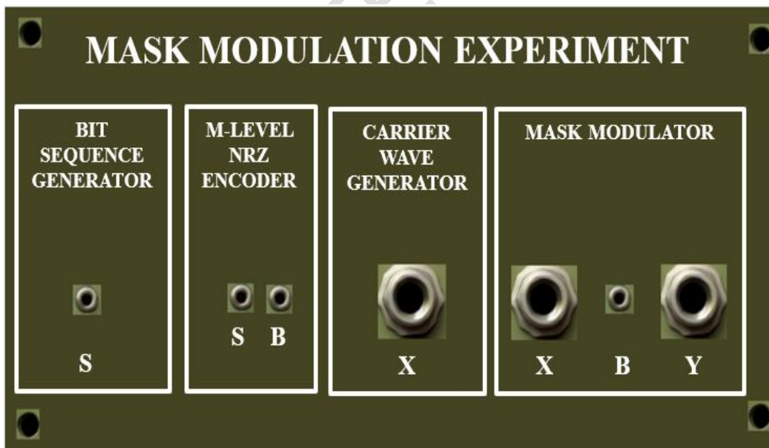
Fig.7. Experimental Equipment for MASK Modulation
