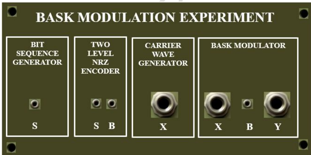
Fig.7. Experimental Equipment for BASK Modulation
