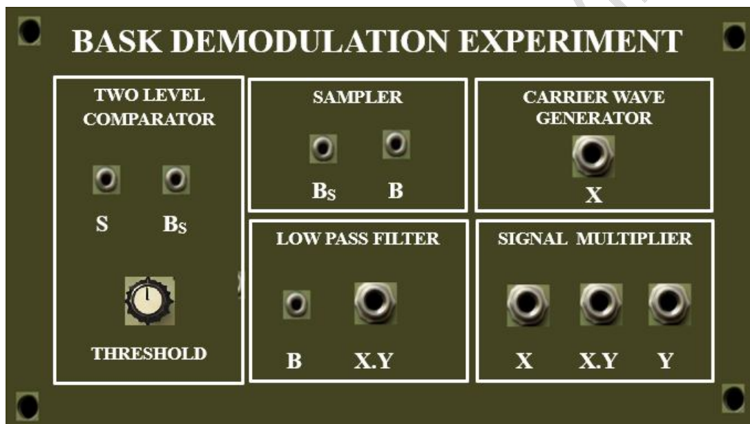
Fig.8. Experimental Equipment for BASK Demodulation
