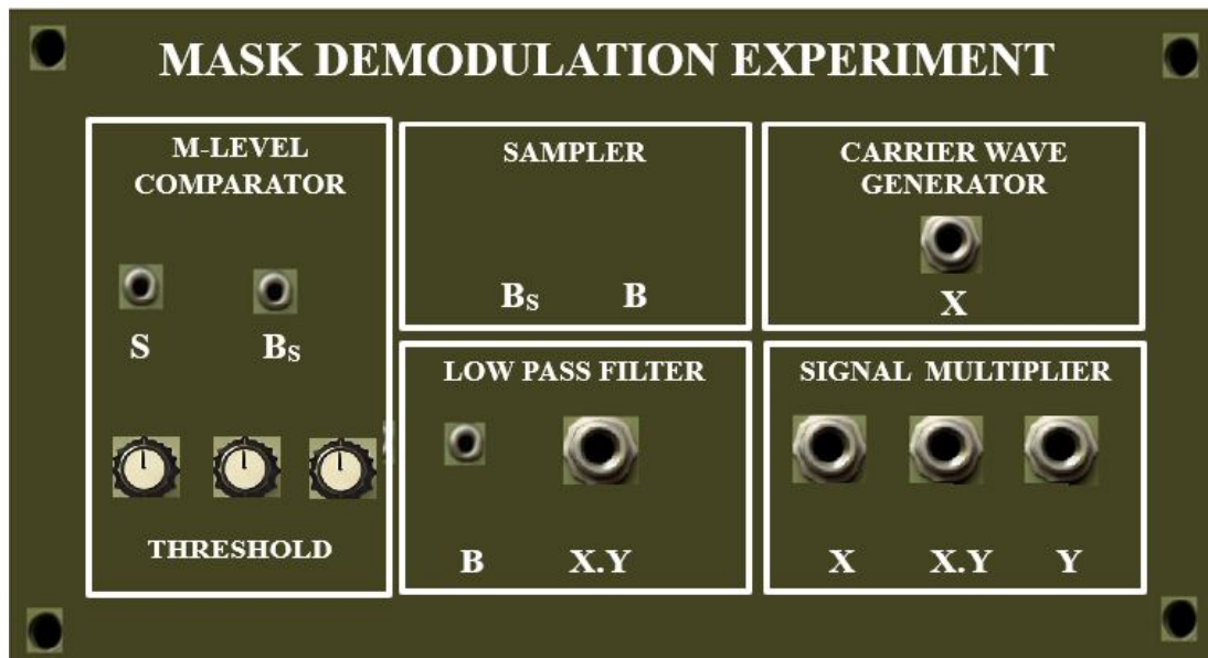
Fig.8. Experimental Equipment for MASK Demodulation
